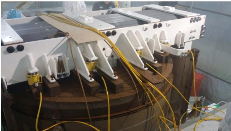
▲ core & coil pressing system by max. 8 hydraulic jacks
